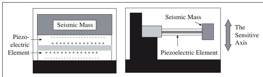
Fig. 1.—Left: Integrated chip sensor. Right: Cantilever beam.
