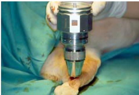
Fig. 1. Extraction of implants from the region tibial of the animals using the torque calibrator (Gauge Tonichi® model BGT150CN-S).
