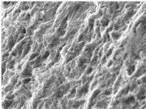
Fig. 2. Appearance of the Defcon TSA® surface under the electron microscope. Note the homogeneous appearance of the roughness.
